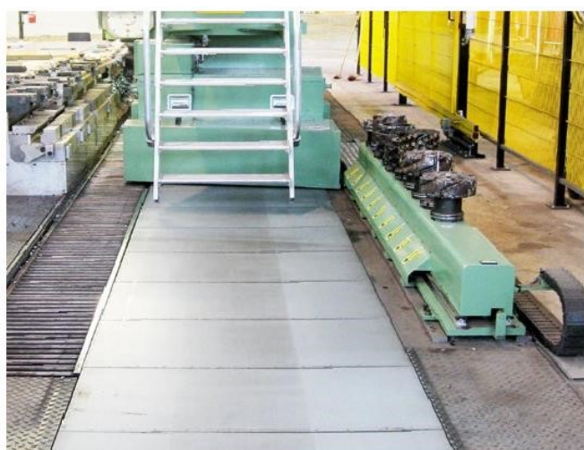
STEELFLEX na vrtačce/ STEELFLEX on a drilling machine
