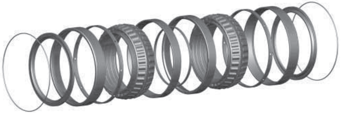
Fig. 45. Sealed roll neck bearing.
