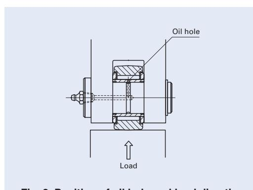
Fig. 2 Position of oil hole and load direction
